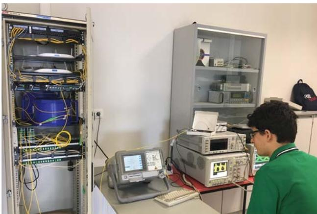
Figure 3. The GPON testbed and the optical instrumentation used in the optical communication laboratory
